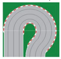
Some simply do not like bottlenecks. For them, it is the 317 and the mirror 318, the second way to get to without a crash around the curves. These modules have taken our standard dimension of 170 x 85 with a format of 121 x 111 $^{\text{th}}$  Run-off areas are directly integrated to a width of 15 cm. The course length (middle lane) is 2288 mm.
