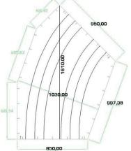
The most important external dimensions in mm. Examples range with the 45-degree turns.
