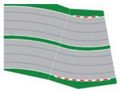
Each track consists of three curve radius. Deputy way open and close the curves. In the narrow sector where outside space for drifting is required, the run-off areas are integrated directly. Therefore, the modules broaden there to 95 cm.
